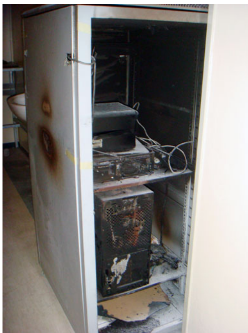
Fig. 2 Suboptimal digital solution: a burnt-out server innovation for a World Health Imaging Alliance-site using a World Health Imaging System for Radiography (WHIS-RAD) with a customised computed radiography (CR) system
