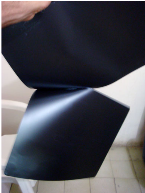
Fig. 5 Problems with wet developing of hardcopy include, amongst other problems, incomplete drying and films sticking together
